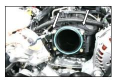
**4.** With a 4mm socket, remove the two studs that held the throttle body to the intake manifold.
