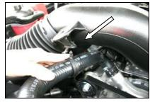
1. <u>Disconnect the negative battery cable!</u> Lift up on the front of the and beauty cover and remove it from the vehicle. Push down on the radiator hose, and separate the tube from the plastic clamp.
